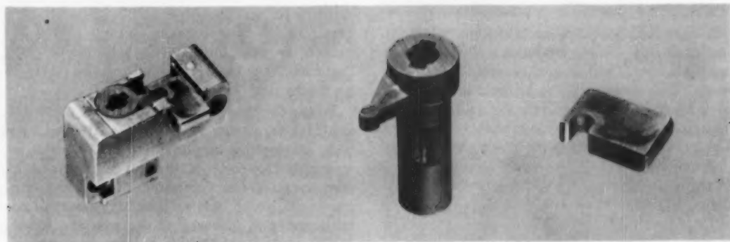
Below: LOCK'S investment cast parts include aluminum housing, 18-8 stainless cylinder and bolt.
